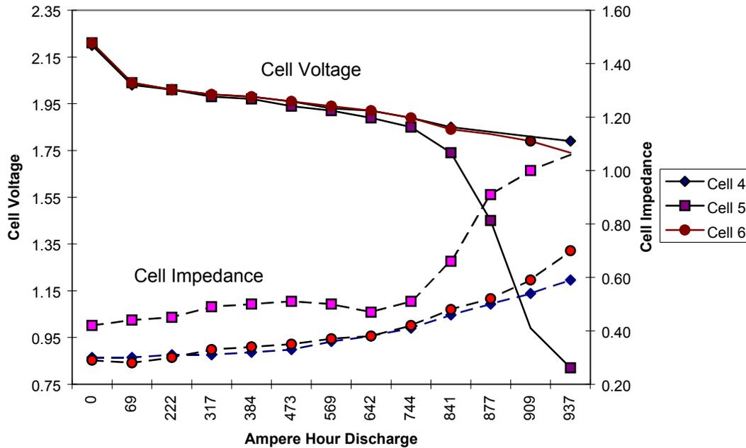
**Figure 6 VRLA Discharge Test Units 4-6**
