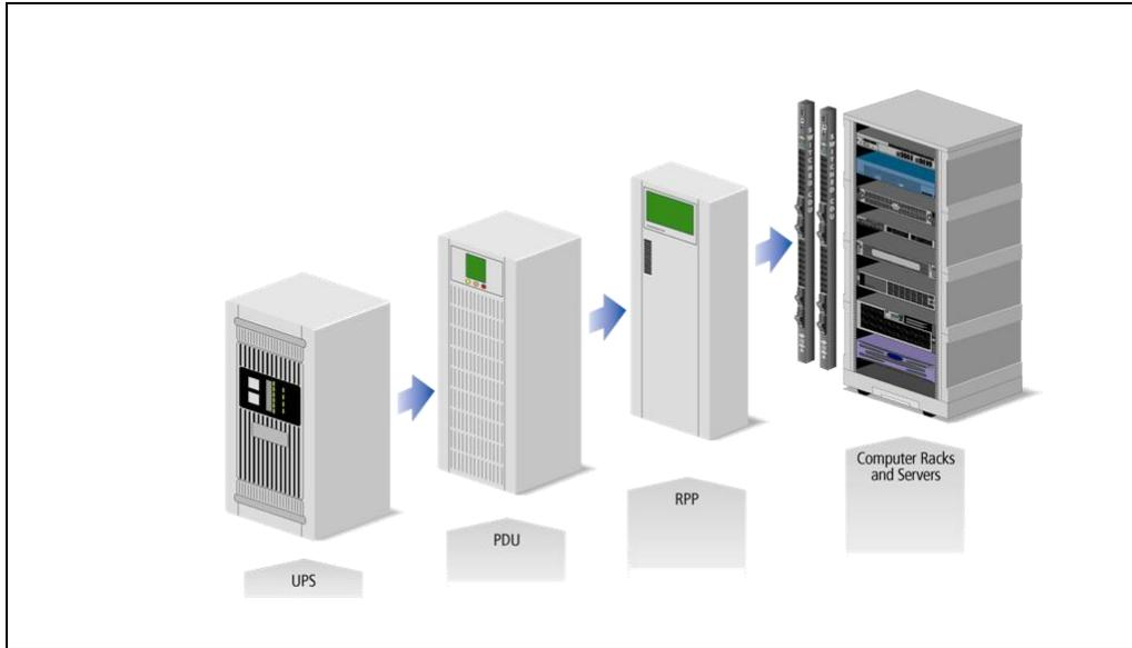
Figure 2: Power Supply Chain to the CDU
