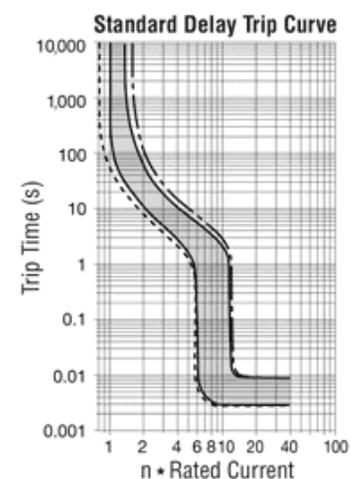
as the threshold current has been reached. This type of delay curve is appropriate for sensitive installations but is not ideal for equipment like servers that typically have inrush currents anywhere from 30 percent to 200 percent above their normal current draw.
