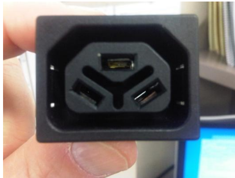
Figure 5, 277V Rated Receptacles The plug shown is close in form factor to the standard C-13 outlet as seen in Figure 6 above. This configuration allows for rapid incorporation into existing PDU form factors while ensuring that existing 208V-240V power cords are not able to plug in.
